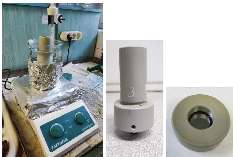
Figure 11 Po-210 source preparation
